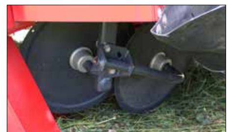
Double swath rollers are standard.
