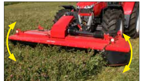
Flexible headstock for perfect ground contour following.
