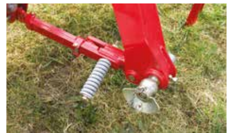
Safety system: Less impact on the cutter bar in case of hitting a big obstacle.
